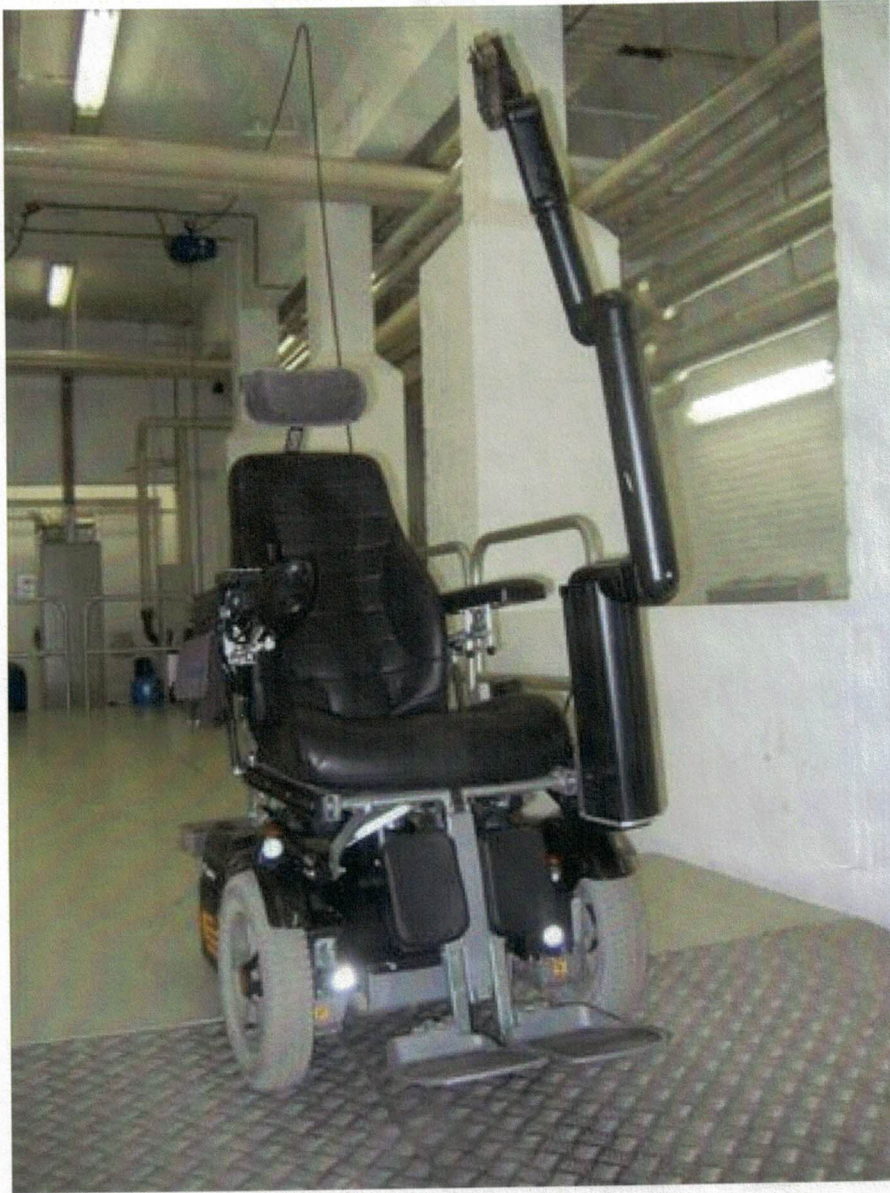
Figure 1: Photograph of the tested sample, trademark: Permobil, type: C500, with robot manipulator trade mark: Exact Dynamics, type: iArm
